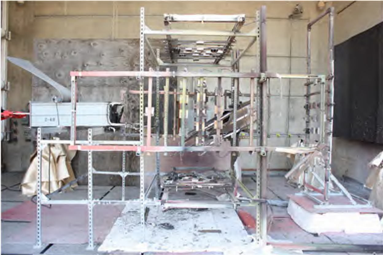
Fig. 202. Post-Experiment 2-40 Bus Duct. Duct severed with a portion resting on the support structure.
