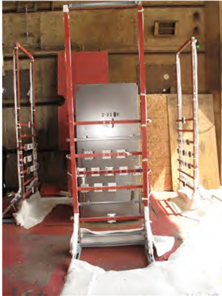
Fig. 165. Pre-Experiment 2-33B. Viewed from side opposite power supply, showing instrumentation rack arrangement surrounding enclosure.
