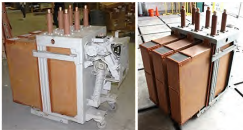
Fig. 14. Photo of AM-7.2-500 GE Magne-blast breaker
