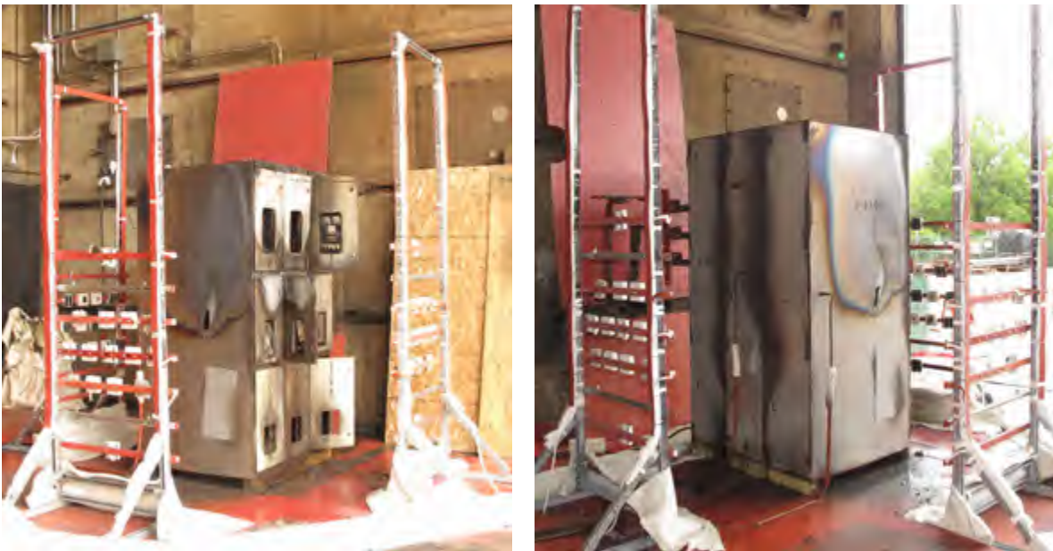
Fig. 167. Post-Experiment 2-33B Left – front corner view, Right – rear corner view.
