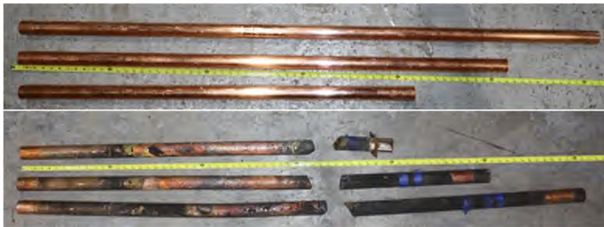
Fig. 56. Photo of Experiment 2-36 bus bars. Top – pre-experiment, Bottom – post-experiment.
