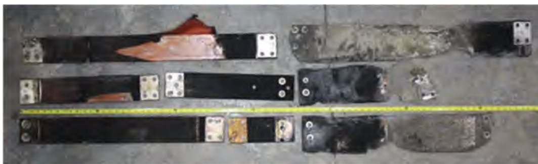
Fig. 50. Photo of Experiment 2-31 bus bars post-experiment (arc location shown right).
