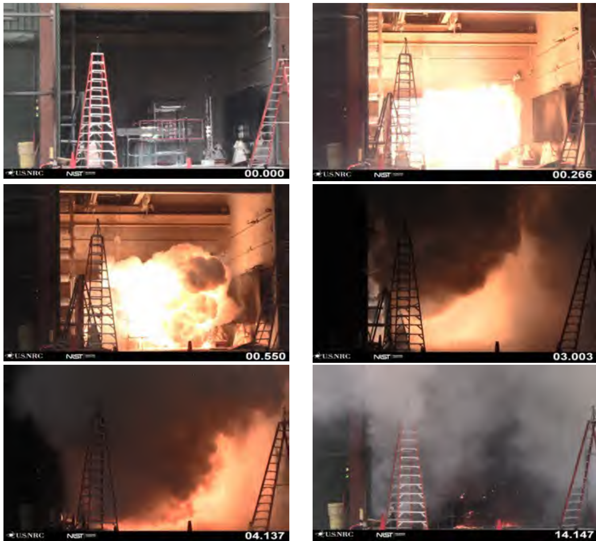
Fig. 84. Sequence of Images from Experiment 2-41 (image time stamps are in seconds).
