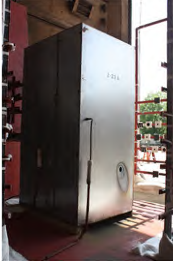
Fig. 32. Enclosures Post-Experiment 2-33A. Note the external breach on the lower portions of Enclosure 'C'.
