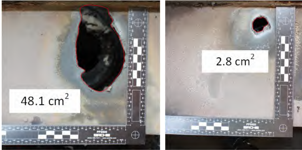
Fig. 195. Post-Experiment 2-38 Internal Breaches Enclosure "L".
