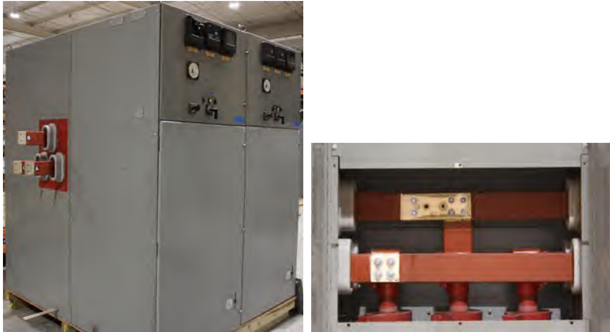
Fig. 186. Pre-Experiment 2-37 Enclosures “J” and “I”. Left – off angle view of Enclosure “J” (left) and “I” (right), Right – arc location main bus.
