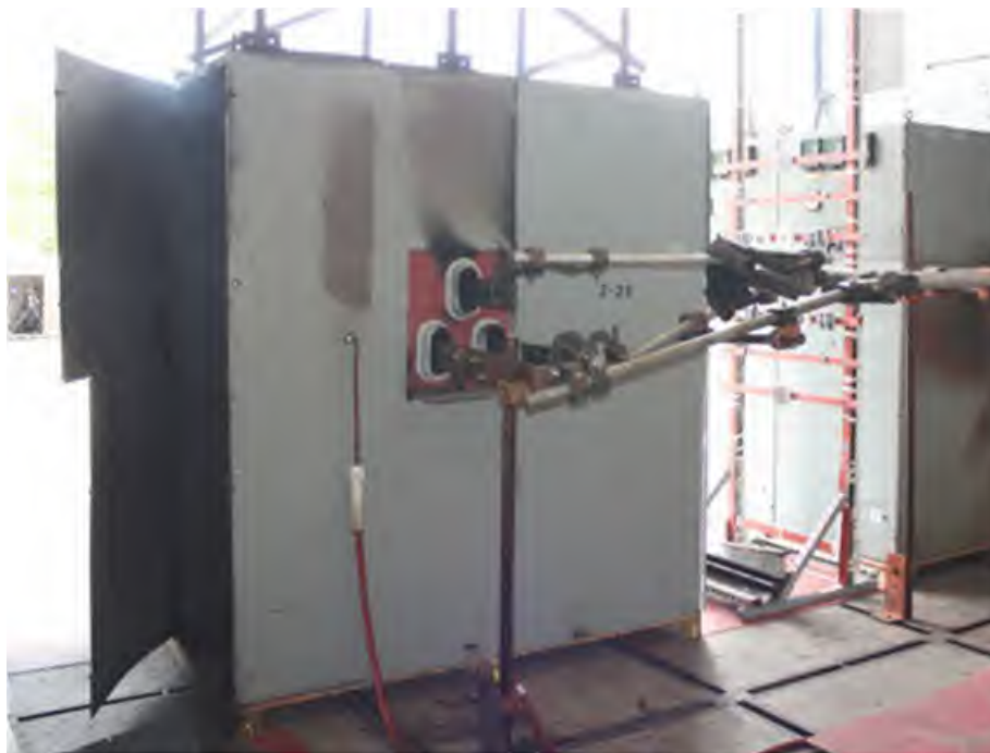
Fig. 69. Enclosure Post-Experiment 2-38. Enclosure “K” is in the foreground attached to the laboratories power supply, Enclosure “I” is across the aisle from “K”.
